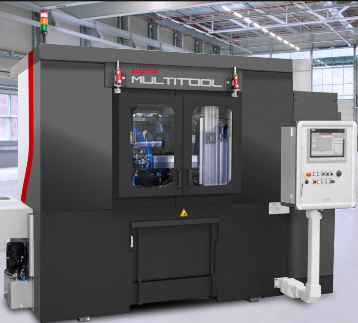
Flexible superfinishing of shafts
