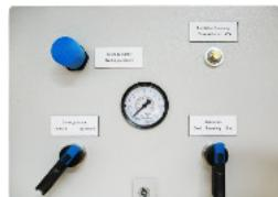
**Pneumatic control units** make a remote control of the attachment possible. The cable length is limited to 5 m.
