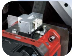
■ Spindle gear box transmission
