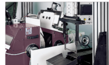
13. Auto. loading and unloading attachment (infeed grinding)
