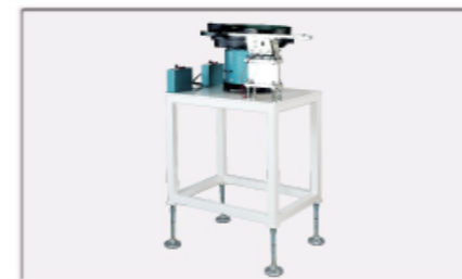
14. Vibratory feeder (thrufeed grinding)
