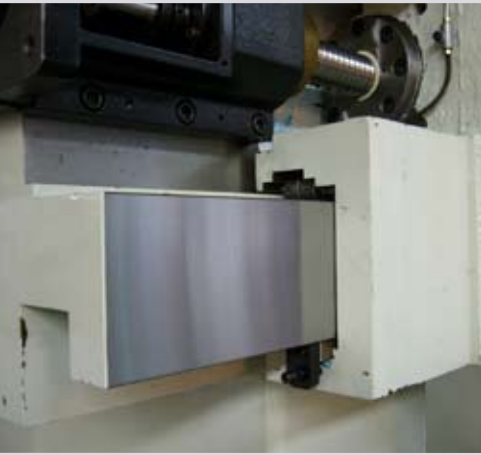
Slide ways design for both rigidity and accuracy,兼顾鋼性與精度。
