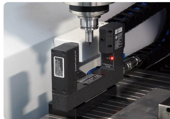
CWM-540G 雷射刀具校正 The Tool Compensation by Laser
