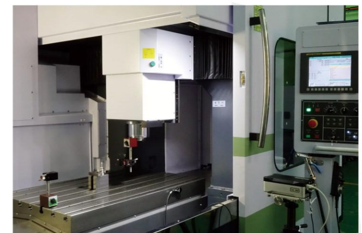
雷射校正 Laser interferometer calibration
