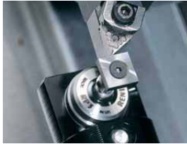
Tool setter provides quick and easy tooling set up (opt.)
